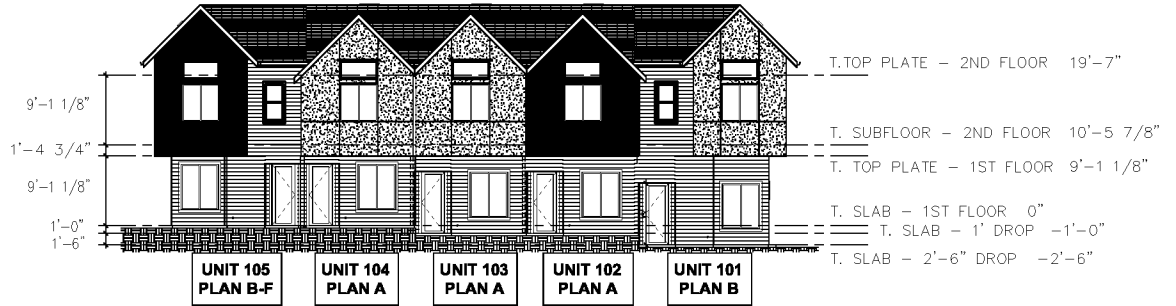
BUILDING 1 FRONT ELEVATION
