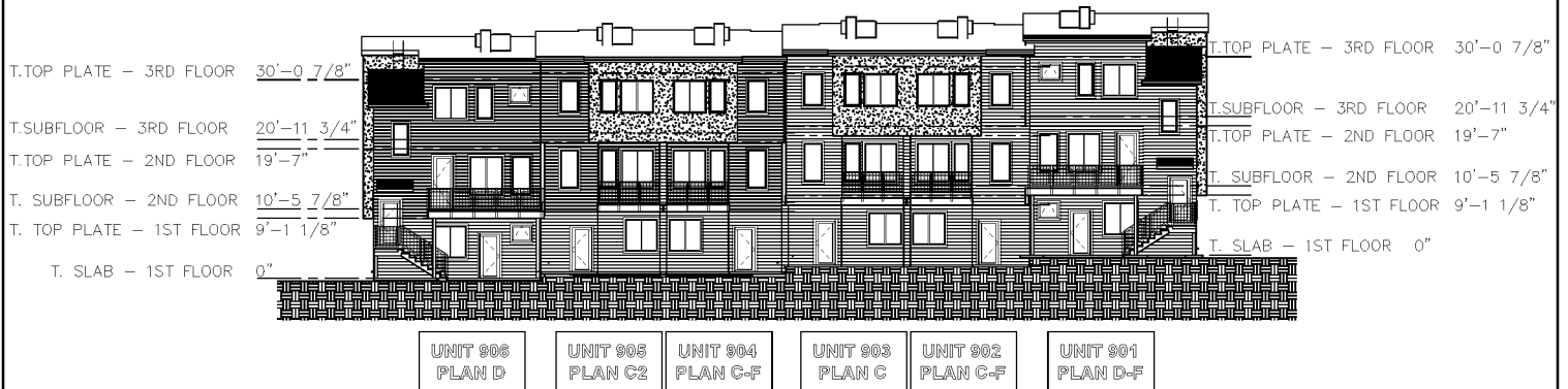
BUILDING 9—REAR ELEVATION
