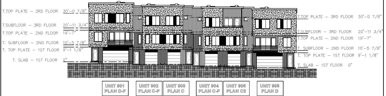
BUILDING 9—FRONT ELEVATION
