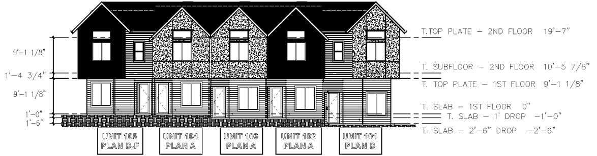
BUILDING 1 FRONT ELEVATION
