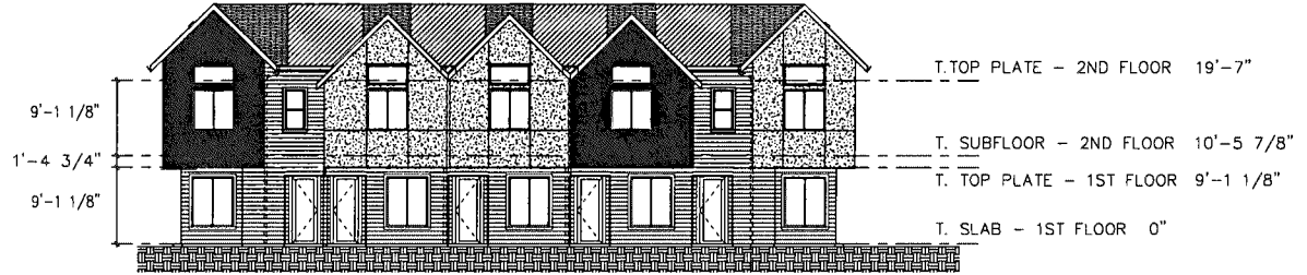
BUILDING 3 FRONT ELEVATION
