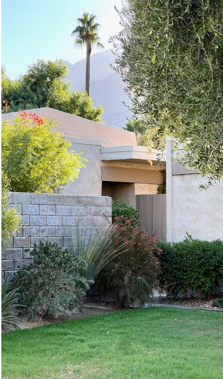
A 2024 image shows the simple elements — turf, plantings of varying heights, slumpstone walls, troweled stucco, shade overhangs, Douglas fir horizontal accent strips, flat rooflines with metal flashing, rooftop HVAC enclosures, wooden gates, recessed entryways — used by architect Donald Wexler to compose pleasing volumes in tune with the desert and mountains. (Photo by Claude Peck)
