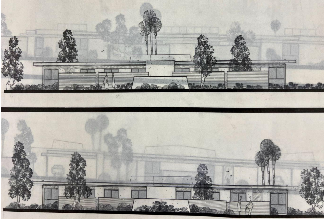
Two 1972 drawings by Wexler show the trapezoidal trash can enclosures (center) and rooftop enclosures for HVAC. Also visible: the two heights for slumpstone patio walls; six feet (top) and 4½ feet (bottom). The full-height windows shown at far right and far left were reduced to half-high ones, at the corners of the 3-bedroom units, possibly as a cost-saving measure. (Original drawings courtesy of Wexler archive, CalPoly Pomona)
